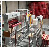
robot-stacker combination was specially designed and built to increase the rate of production and the overall quality of the full pallet. A special metal detector on the input line checks for the presence of any metal parts inside the bag, plus a checkweigher ascertains whether the bag complied with weight limits set by the customer, with the automatic rejection of any non-compliant bags.
